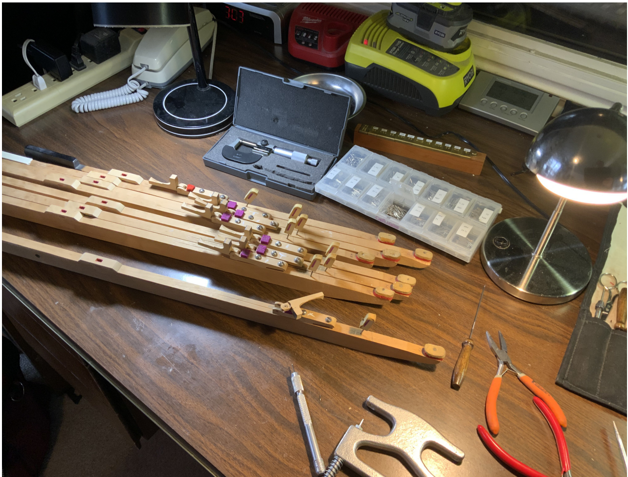
Repairing Jack/Wippen Cord & Spring Regulating
