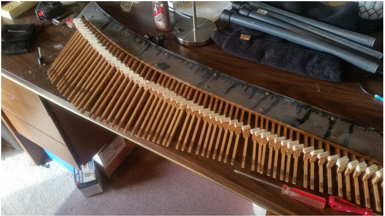
Repairing Damper Blocks, and Dampers
