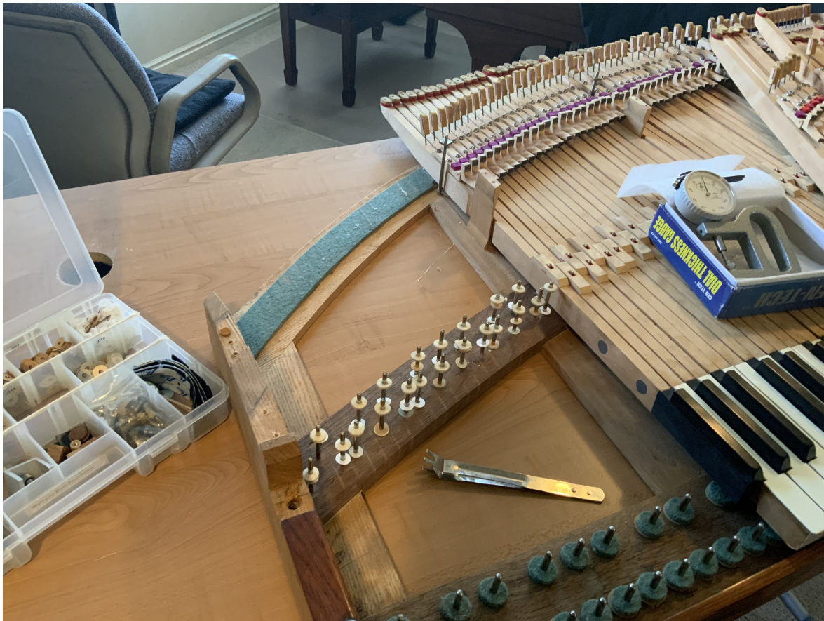
Leveling White Keys Adjusting Key Travel
