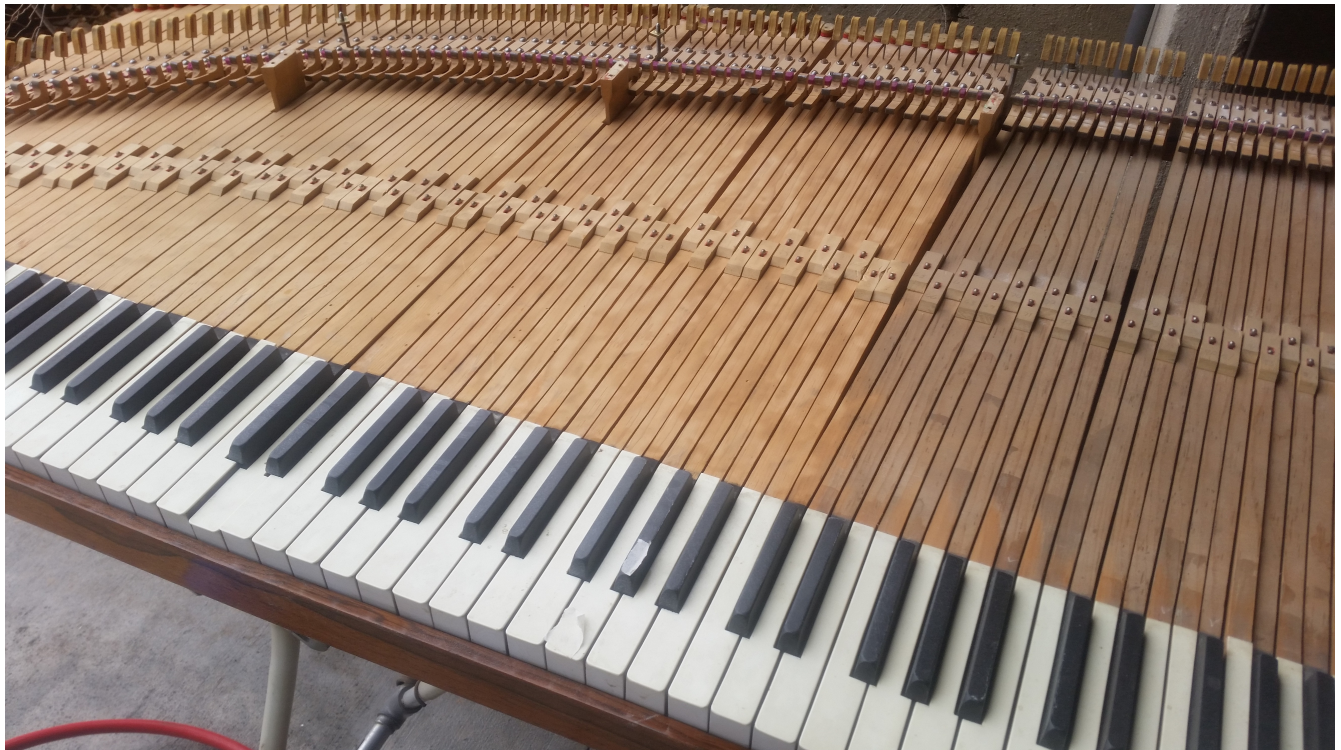
Deep Cleaning Keys, Piano Cavity, Soundboard (under strings), Key Sticks, Balance and Front Rails, Action, Catchers, Various Felt Rails, Buttons and Damper Mechanism
