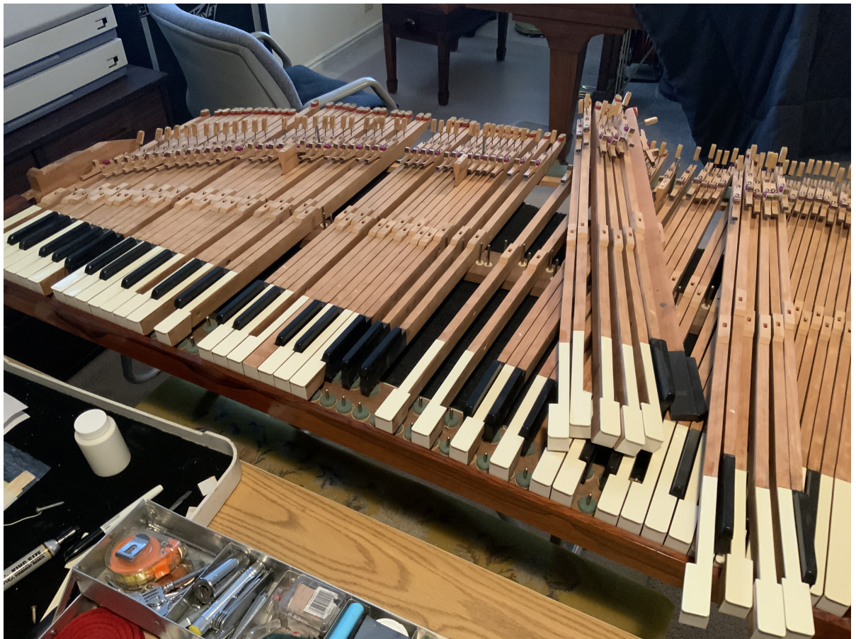
Reaming Key Hole Spacing and Mortise (1/8")... Easing Bushings, Repair and Adjustments.
