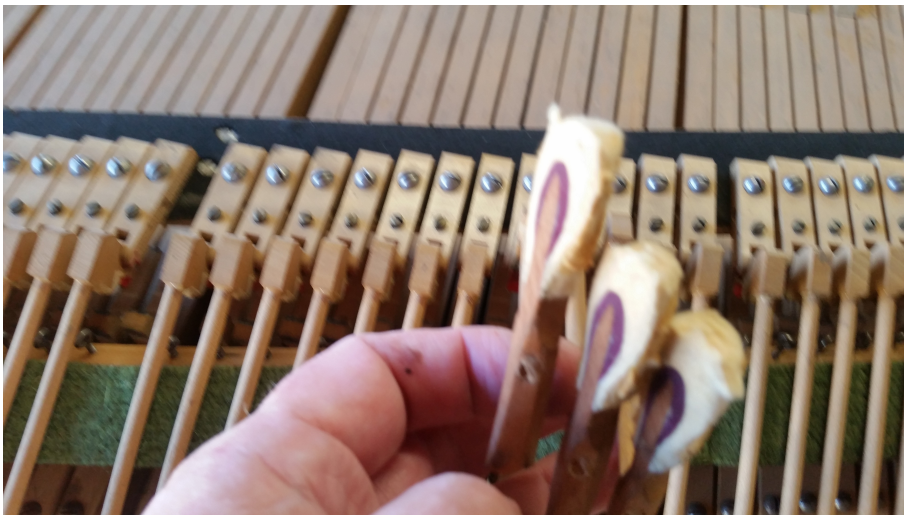
Evaluating Hammers and Possible Repair Solution..
